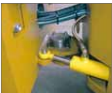
Unique pivot articulation with grease point
