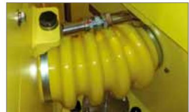
Double articulation with lubrication points 'Pac-Pivot' (patented)
