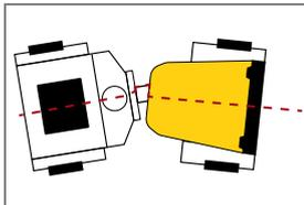
The shape of the roller provides high visibility around the edges of the rollers during operation.
